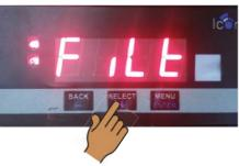
Push "MENU" X 21 to adjust the software damping filter.
