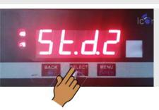
Push "MENU" X 11 to adjust relay 2 start up delay.
