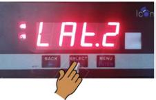
Push "MENU" X 14 to enable relay 2 latch point.
