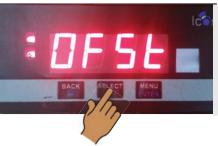
Push "MENU" X 18 to display the off set. When "OFSt" is displayed, push "+" or "-" to 0.0V
